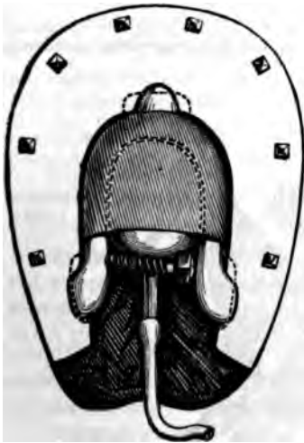
FIG. 175.— Chaussure exploratrice , or pneumatic foot-bulb of Marey, for the registration of the gaits by compressed air.
